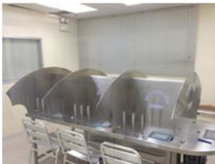
Figure 3: Olfactory Laboratory with Scentroid™ SS600 Olfactometer
